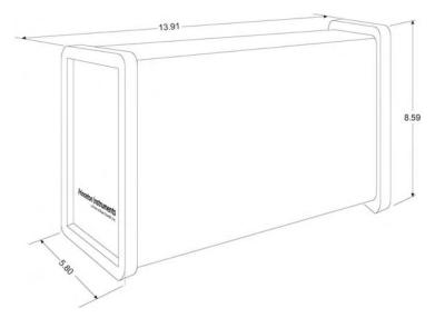
Figure 42. ST-133B Controller Dimensions
